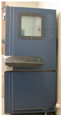
Diag. 7: Climatic chamber
